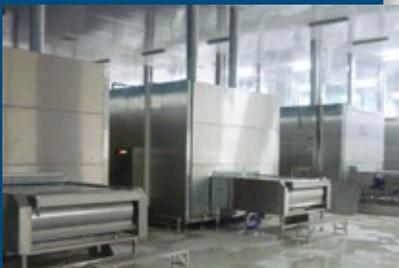
▲ The fish filets have to be individually quick frozen to ensure freshness and highest quality of the finished goods. Guntner's stainless steel GCO heat exchanger coils enable this high tech process.
